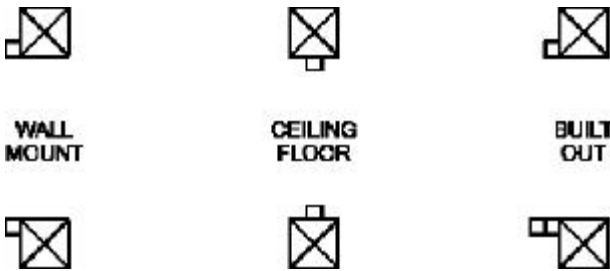
FIGURE 1 THREE (3) BASIC STORM PANEL ATTACHMENTS FOR TESTING.
